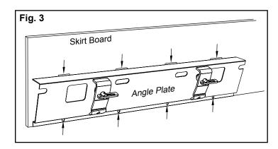
**Step 3. Weld the angle plate to the skirt board.** Stitch weld top edge with 6mm (1/4") weld, 50mm (2") long, in at least 4 places. Plug weld bottom edge 4 places in holes provided (Fig. 3).
