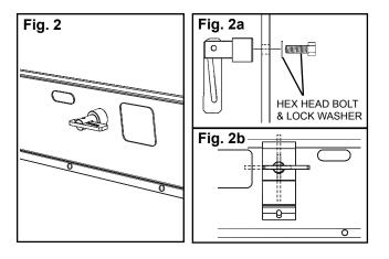
**Step 2. Mount two clamp pins to the angle plate.** Screw hex head bolts and lock washers through the angle plate into the clamp pins and tighten securely (Fig. 2, 2a). **NOTE:** Determine the best direction the wedge in the clamp pin should be in for easy access (Fig. 2b). Once the pin is bolted to the skirt board the wedge direction is fixed.
